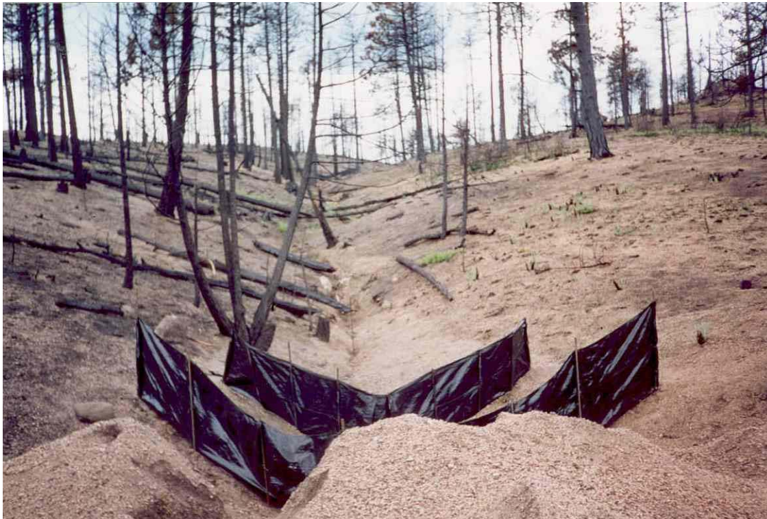
Figure 4. A pair of sediment fences used for measuring hillslope-scale sediment yields after the June 2002 Hayman fire. The piles of sediment are the material captured and removed from the fences between July 2002 and early summer 2003. This area burned at high severity, and the slow recovery is evident from the small amount of vegetative regrowth.
