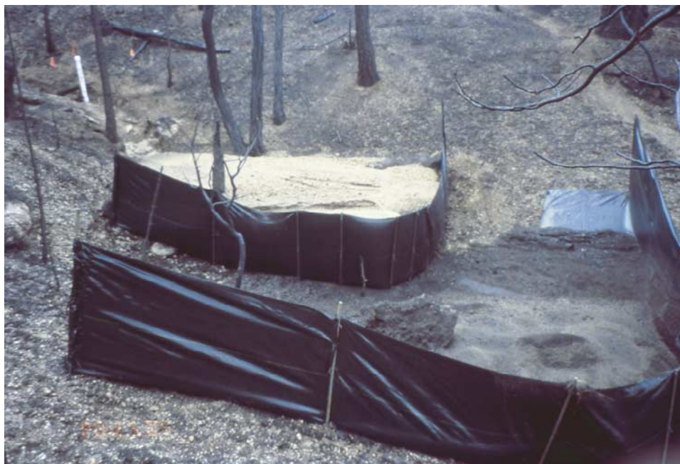
Figure 2. A typical set of sediment fences used to measure sediment yields from a convergent hillslope. Photo taken 1 month after the Hayman fire.
