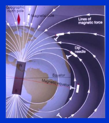
The direction and inclination in which a dip-needle points reflects the earth's magnetic field:-
