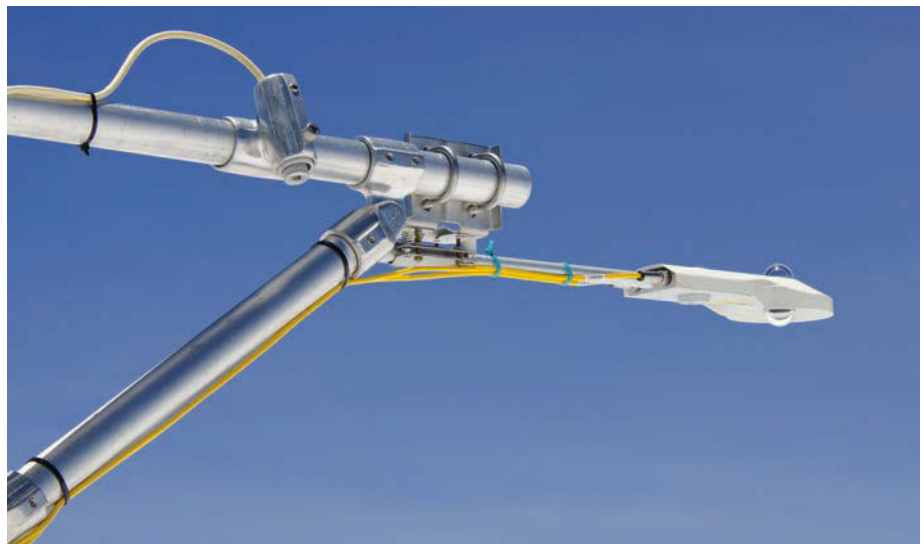
Figure 5: The net radiometer and infrared temperature transducer installed on Kilimanjaro in October 2012 both view the same area of glacier surface
