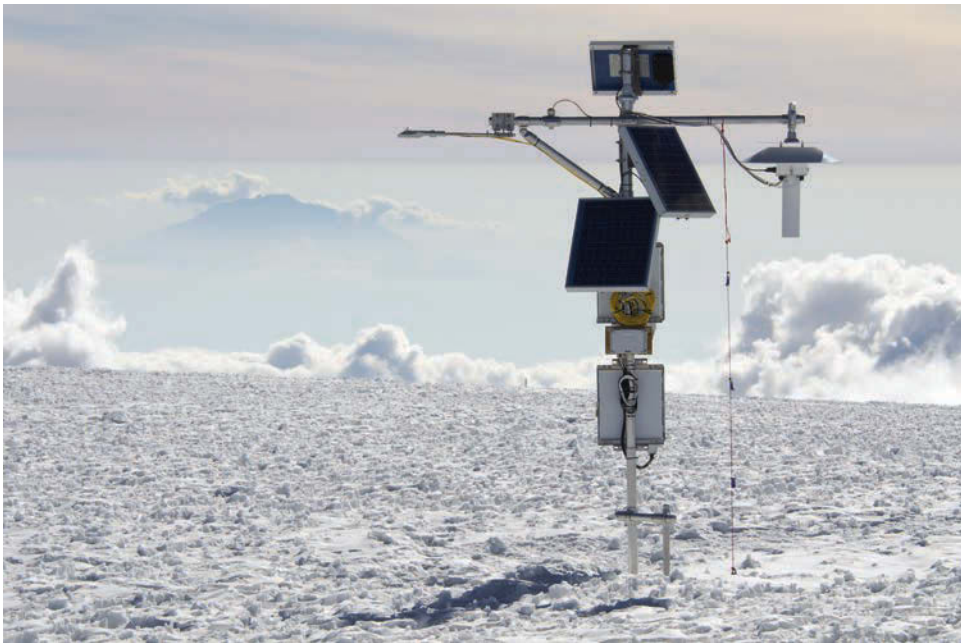
Figure 4: This AWS on Kilimanjaro's Northern Ice Field at 5,775m has a net radiometer (left-hand side) and fan-aspirated shield for a temperature and humidity sensor (right). Mt Meru, 70km away, can be seen in the background
