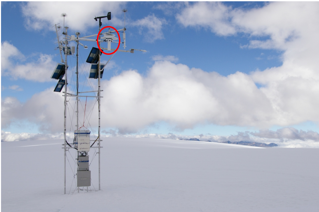
Figure. Quelccaya Ice Cap automated weather station at \sim 15:00 local time on 4 June 2010. Air temperatures are measured in the white shield, here highlighted within the red oval. The lower of the two upper shielding disks is 51 cm in diameter. Measurement height at the time was \sim 4.5 m. This view is looking approximately to the northeast.
