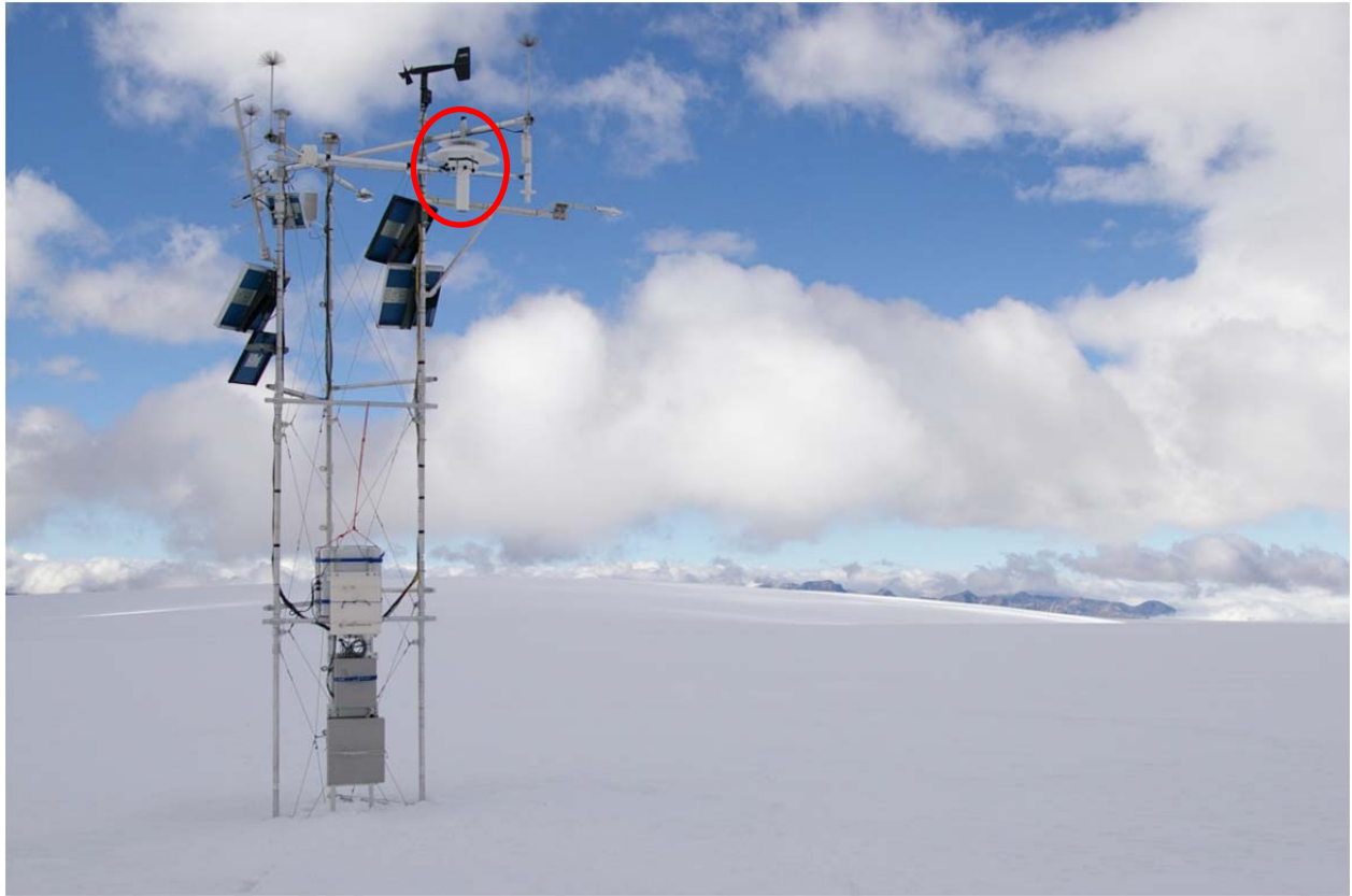
Figure. Quelccaya Ice Cap automated weather station at ~15:00 local time on 4 June 2010. Air temperatures are measured in the white shield, here highlighted by within the red oval. The lower shielding disk is 51 cm in diameter. Measurement height at the time was ~4.5 m. This view is looking approximately to the northeast.
