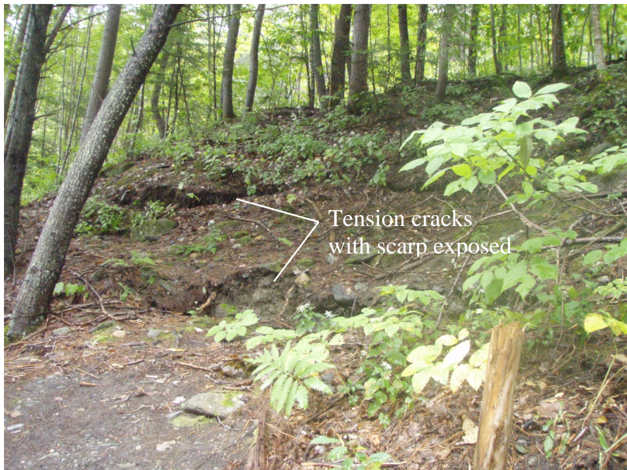
Figure 12. Tension cracks in soil downgradient from roadway at Slide 1. Note bend in tree trunks at top of slope indicating slope instability.
