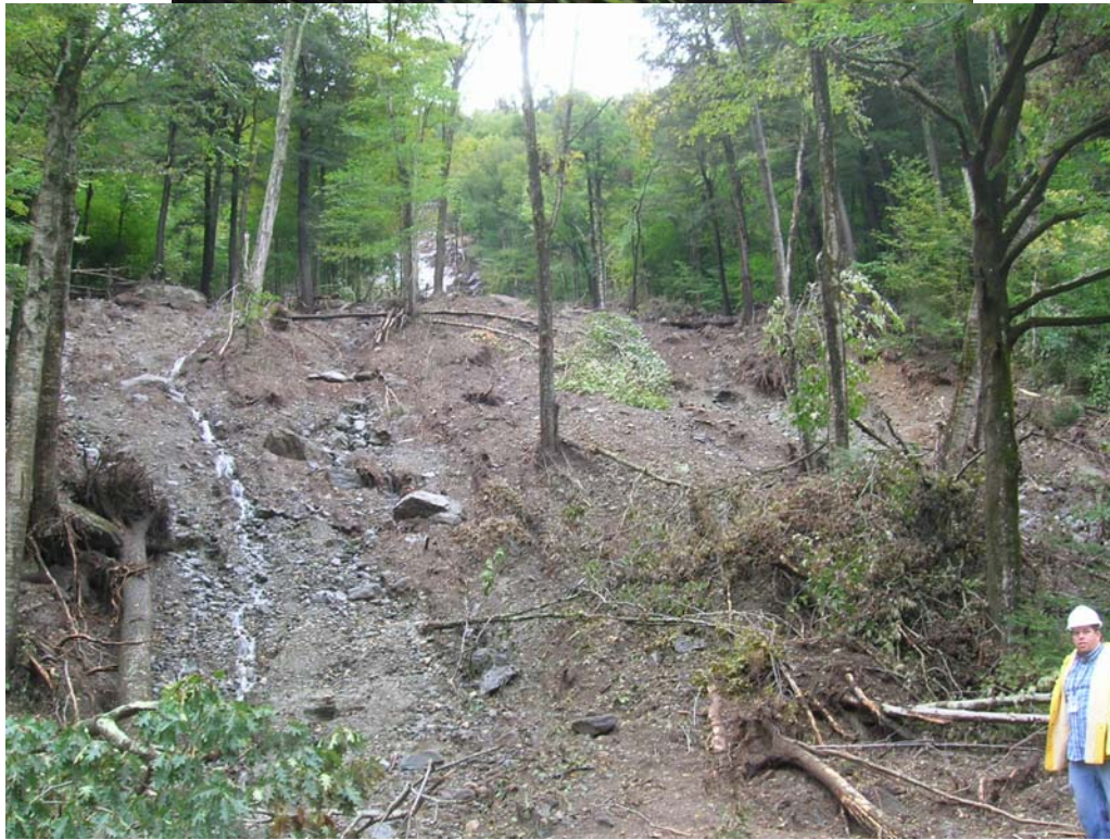
Figure 7. Upper figure is a google maps image showing the approximate location of slides 2, 3 and 4 (yellow outline). Note the bench in slope near slide. In lower figure bench is evident by break in slope near top of picture. Bedrock sheeting joint is exposed in distance. Debris avalanche slid off the sheeting joint surface as a translational slide then flowed up and over the bench before spilling out on to the roadway. Laminated sediments exposed in gulley to right. Photo by Joe Kopera.
