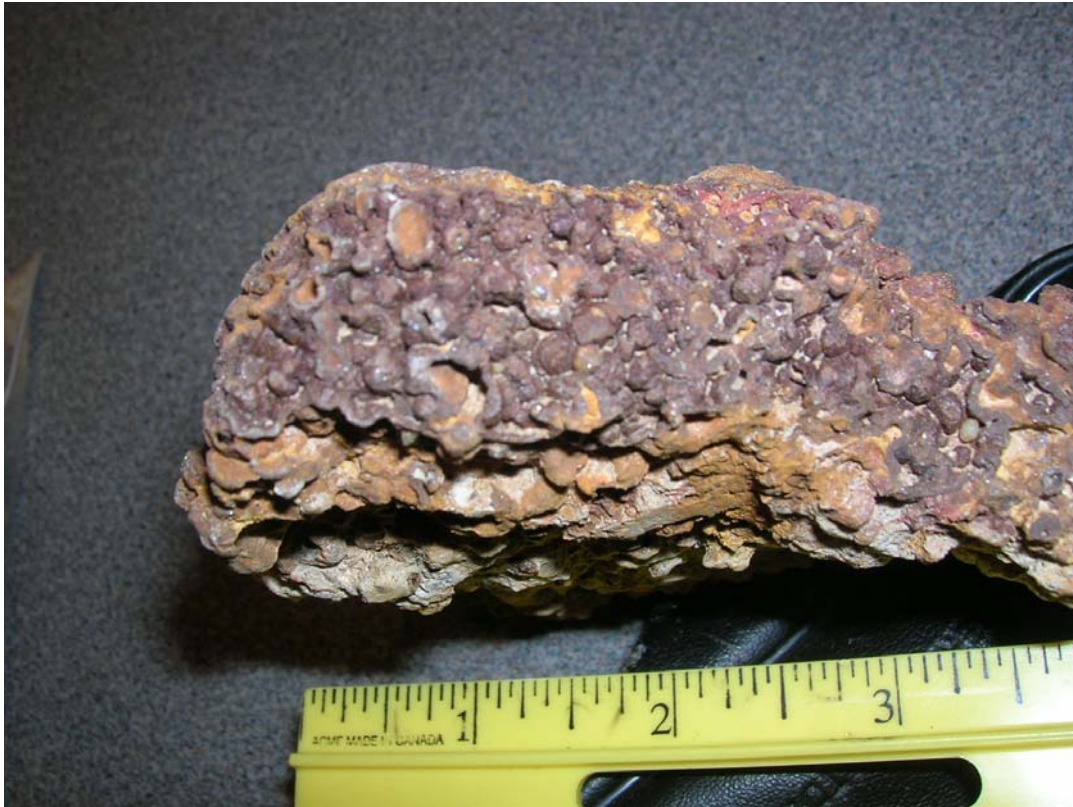
Figure 12. Example of iron-rich rock showing pisolitic texture. Spherical pisolites are 1 to 1.5 cm in diameter.
