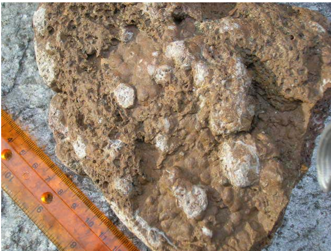
Figure 11. Sample of iron-rich material showing the characteristic botryoidal (grape-like) texture (see lower part of sample at 6 o'clock). Sample was collected by the Trustees of Reservations and was the sample analyzed with the scanning electron microscope. Ruler for scale.
