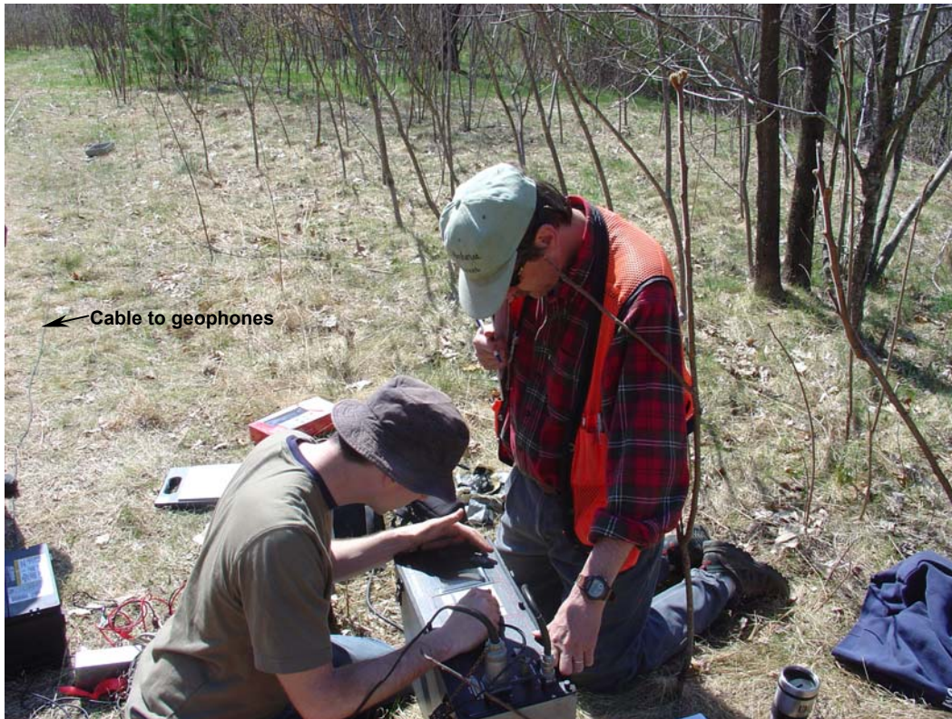
Figure 6a (top). Picking the arrivals times of p-waves on the seismograph.
