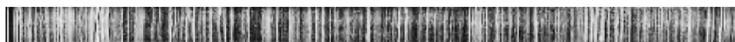
Fig. 5. A linescan image of NGRIP ice core interval 2528.35–2530.0 m depth. Gray layers, annual cloudy bands; annual layers are about 1.5 cm thick. Age of this interval is about 72 ka, which corresponds with Greenland Interstadial 19. (Svensson et al., 2005) [Copyright 2005 American Geophysical Union, reproduced by permission American Geophysical Union].
