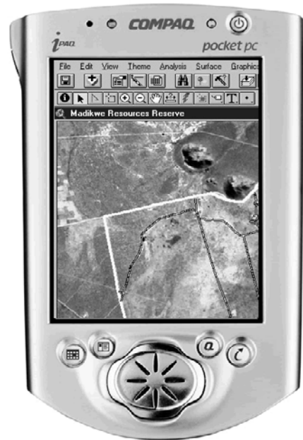
Figure 1-7: Portable computing is one example of the technological pull driving GIS adoption. These hand-held devices substantially improve the speed and accuracy of spatial data collection (courtesy Compaq Computer Corp.).
