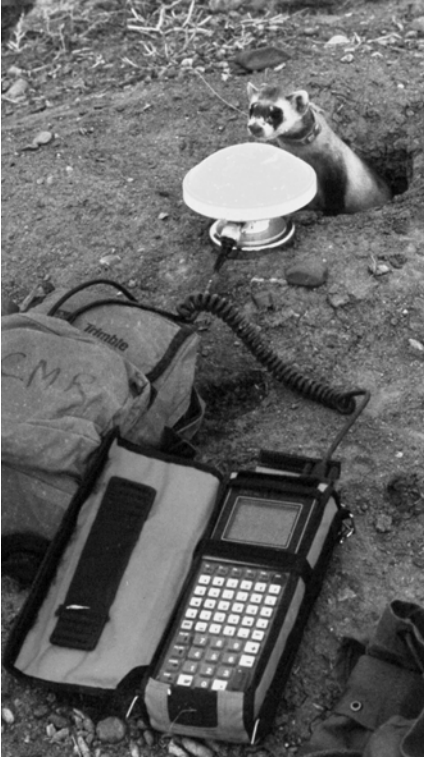
Figure 1-12: Specialized equipment is used to collect spatial data. Here a burrow location is recorded using a GPS receiver, as an interested black footed ferret looks on (courtesy Randy Matchett, USFWS).
