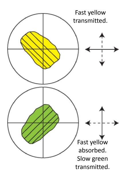
Plane polarised light is vibrating in one plane (E-W).
