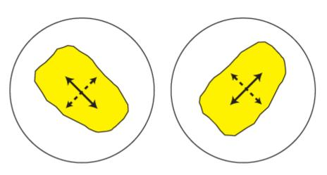
By using an accessory plate (commonly gypsum or quartz) it is possible to artificially augment or hinder the retardation.
