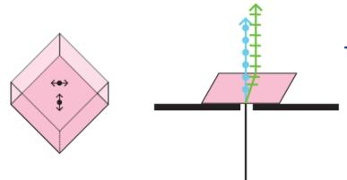
The RI of a mineral varies as a function of the crystallographic axis (orientation of C) such that the two beams are created simultaneously but exit at different times.
