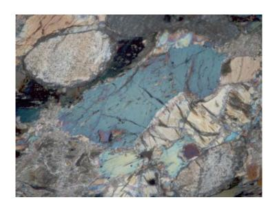
When **monochromatic** polarised light enters an anisotropic mineral it splits into perpendicular components creating two light beams that are independent.
