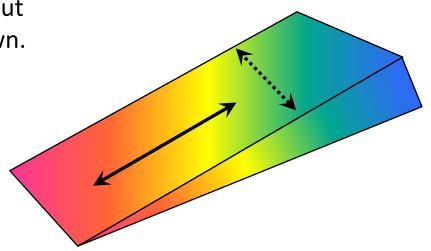
When the accessory plate augments the retardation (i.e. increases the path difference) the order of birefringence colour increases.
