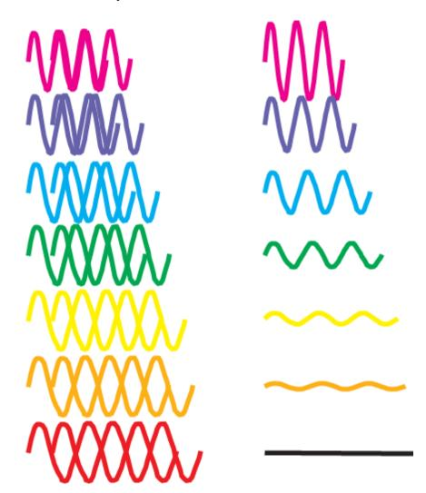
Retardation holds back particular wavelengths. In this case, the red light has been held back ~½ l.
