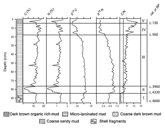
Figure 4 Litho-stratigraphic plot of percentage carbon and nitrogen,  $\delta^{13}$ C,  $\delta^{15}$ N and the C/N ratio from INDRE-C. The vertical dashed line (C/N ratio) indicates the boundary between algal and terrestrial dominated productivity (Meyers and Lallier-Vergès, 1999)
